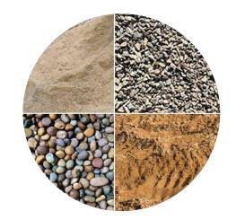
Asphalt is made up of a mix of 95% aggregate material (stone, sand, and gravel sourced from quarries like Canyon Rock) and 5% asphalt cement, the black "glue" like substance that holds the material together
